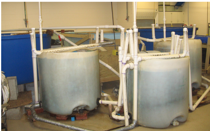
Figure 9. New lab with three biofilters (white tanks on left) and three 600-gallon production tanks (round blue tanks, right foreground, and center background).
