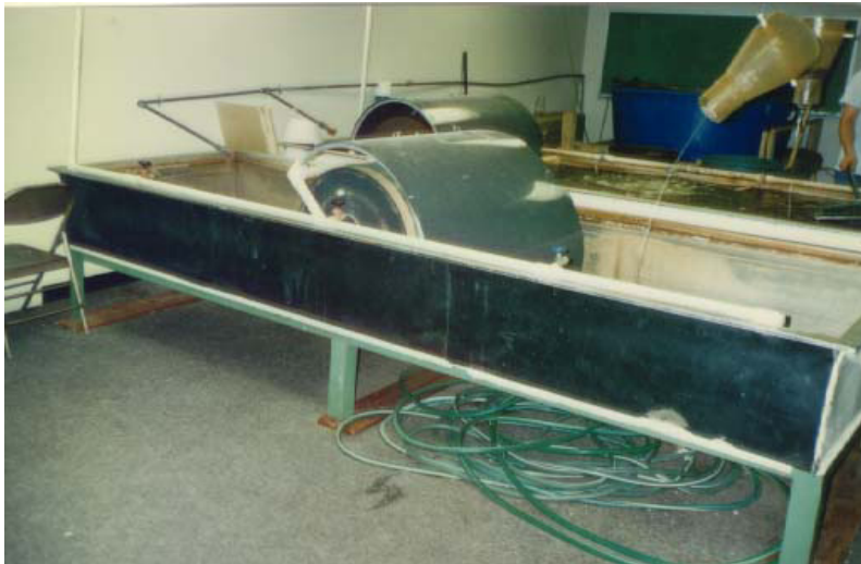
Figure 5. Our first makeshift recirculating aquaculture system (RAS) built with donated stainless steel cheese vats.
