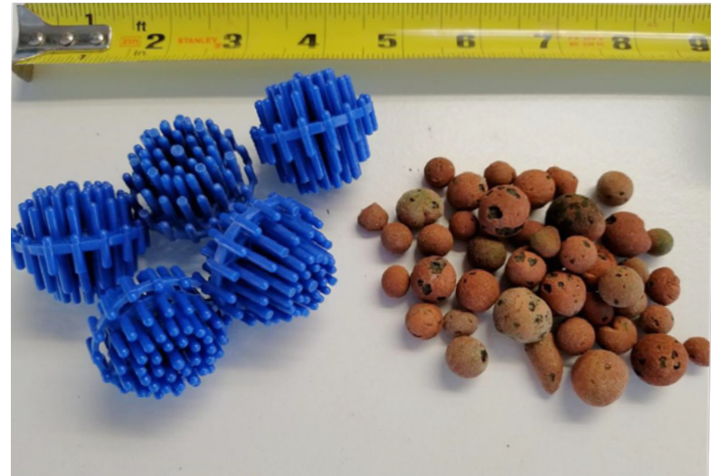
Fig. 6. Examples of biofilter media. (P. Wilborn, 2020.) Aggregates, pea gravel and sand (left); polyethylene Hydroballs and clay Hydroton (right).
