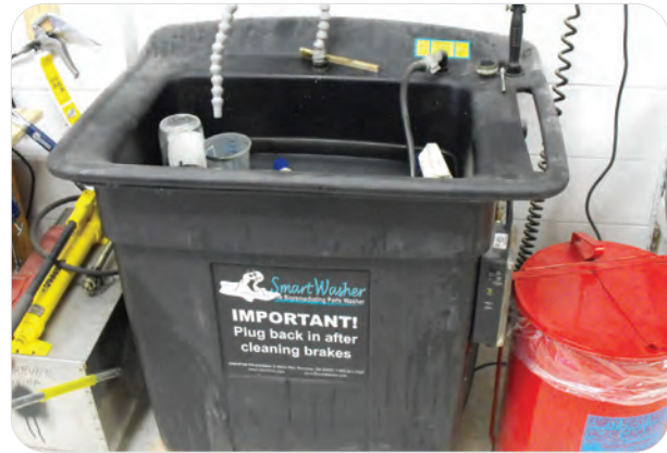
Bioremediating parts washer at Washburn Marina. Photo credit: Gene Clark, Wisconsin Sea Grant.
