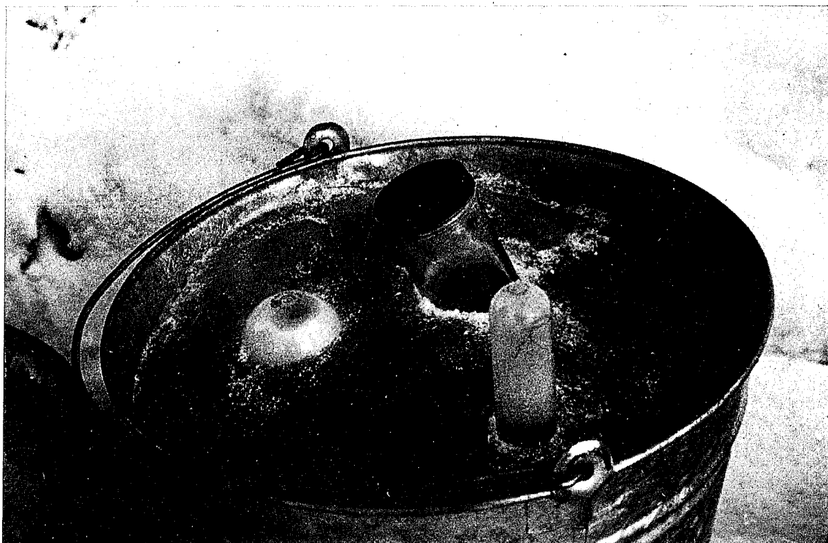
FIGURE 9.2: Glass Objects Subjected to Ice Pressure Squeeze
