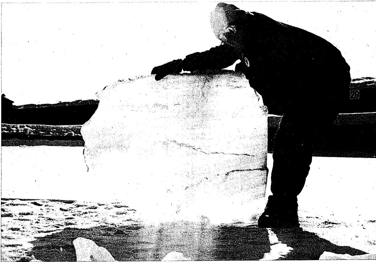
FIGURE 2.2: Ice Cross Section Showing Variability of Ice Sheet
