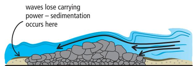
**Tripping Waves (Submerged Breakwater)**
