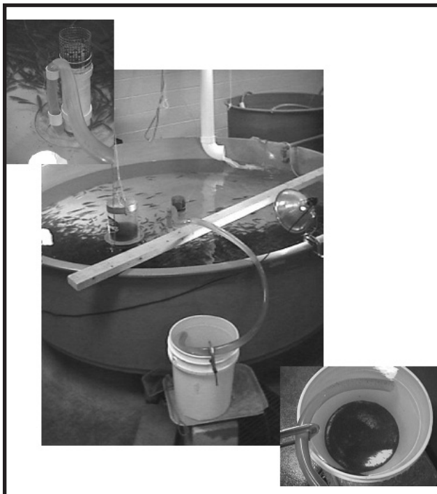
Figure 4. Low head siphon used to gather nearly intact feces and unused food from circular flow-through rearing tanks for use as worm food. Tank inflow was oriented to cause a circular flow in the tank, sweeping settled waste to the central sump. The tank sump was modified (upper left) with a concave poly resin insert that eliminated the right angles of the outer sump wall and permitted waste to accumulate next to the central standpipe. The inflow end of the clear vinyl siphon hose was attached to the standpipe with close fitting rings of PVC. The outflow of the siphon was adjusted to a low velocity by raising or lowering the collection pail (lower right) to just slightly below the water-level of the rearing tank effectively removing the waste intact. The continuous overflow of the collection pail was diverted to the floor drain. Pails of settled waste were periodically exchanged with the bulk of the water decanted and the remaining biosolids used as worm food.
